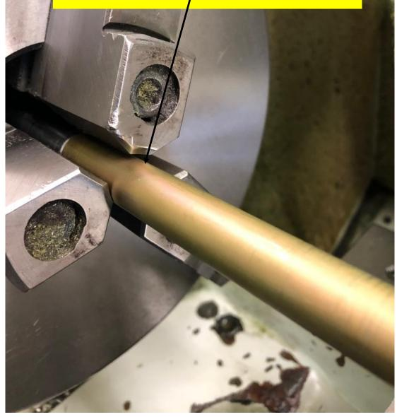
INSERT SPRING CYLINDER ASSEMBLY AND APPLY LIGHT PRESSURE WITH TAILSTOCK. THE SPRING IS UNDER LOAD. DRIVE OUT #12 WITH 3/16" ROLL PIN PUNCH. USE TAILSTOCK ADJUSTMENT TO RELEASE PRESSURE AFTER #10 SPRING PIN IS REMOVED
