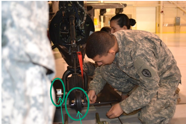
Tail ski with L20500A-14-2 Tow Bar Adapters reinstalled and L20500-18 tail wheel assembly being installed.
