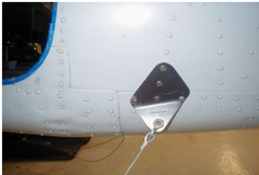
Rear Rigging Bracket Installation LH3600-17 (LH3600-18 Opposite) Photo 2
