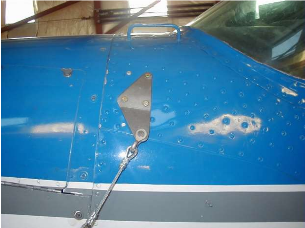
LW3600-180A-9 Forward Rigging Bracket Installed (LW3600-180A-10 is opposite) Photo 1
